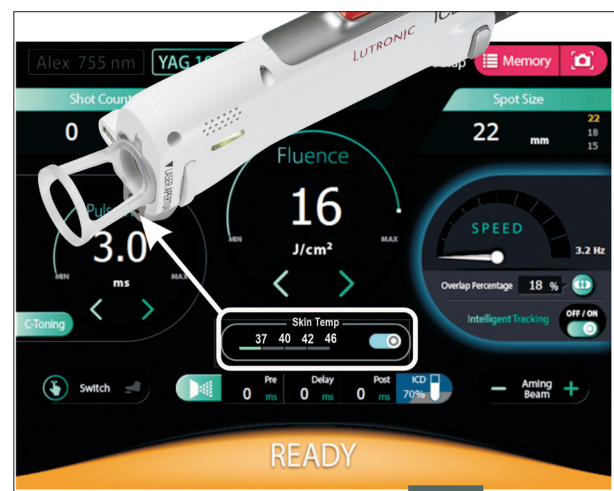
Fig. 2. The GUI (touch screen) of the long-pulsed Nd:YAG laser used in the present study with the skin temperature indicator (white bounding box) and the infrared temperature sensor indicated on the superimposed handpiece (white arrow) (Courtesy, Lutronic Corporation, Goyang, South Korea).
